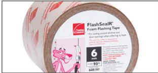
**FlashSealR® Tape:** Flashing tape that helps to provide effective protection against air infiltration and water penetration. Self-adhering without aid of primers and designed to be applicable in cold temperatures. For best adhesion, the tape should be applied over the foam sheathing at the time the sheathing is installed. Thin and flexible to seal around penetrations and uneven surfaces, with aggressive adhesive for long-term adhesion, strength and handle-ability.
